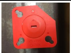
2. Verify correct FMP plate to match coupler. (FMP45 for #4 and #5 and FMP67 for #6 and #7)
