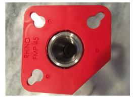
6. Visually inspect the threads to ensure that threads are clear of dirt/debris or concrete. Verify for correct male rebar. Insert and properly torque male rebar into FMP and coupler
