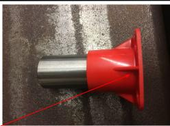
3. Insert coupler into FMP and press fit coupler fully into FMP. Coupler should be flush with FMP base
